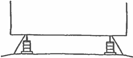
Figure 3 -Recommended Grade Underneath Home
